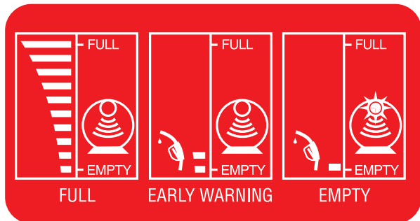
DIAGRAM 3 - Continuous display on small LCD Panel of Receiver 10 bar graph level display
